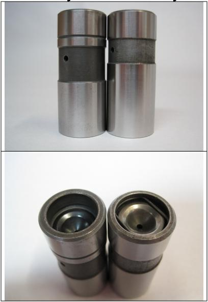
The lifter on the left is a Chevy style lifter which has a much lower oil band than the Pontiac lifter on the right- this will drop out of the bottom of the lifter bore on most Pontiac blocks which will dump oil and could also cause the lifter to "catch" on the bottom of the lifter bore. Also note the different seat height in the Chevy lifter versus the Pontiac lifter (the Chevy lifter requiring a longer pushrod)
